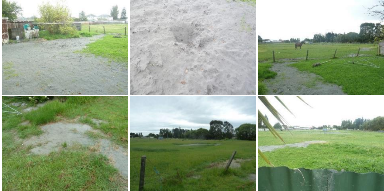
Figure 39: Ground photographs showing ejecta remnants just outside the 20-m buffer, toward the southeast (photograph date: Nov 2011).
