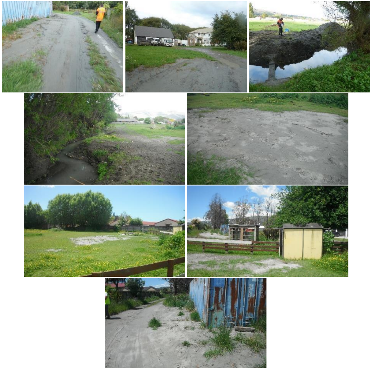
Figure 38: Ground photographs showing ejecta remnants at the property to the north, outside the 20-m buffer (photograph date: Nov 2011).
